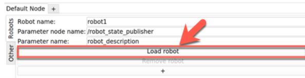
At that point, the robot's model should be loaded and displayed in Slicer. To do this addition programmatically, please see the documentation on the `vtkMRMLROS2RobotNode`. Note that if your robot uses a namespace, you will likely need to prefix this on the parameter node name. The PSM for example requires `PSM1/robot_state_publisher`.
